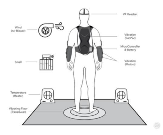
This graphic shows the haptic hardware we use to create the virtual reality tree experiences of movement, air, temperature, and smell.
